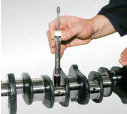
Hardness test with rebound hardness tester (item no. 50 009 812)
