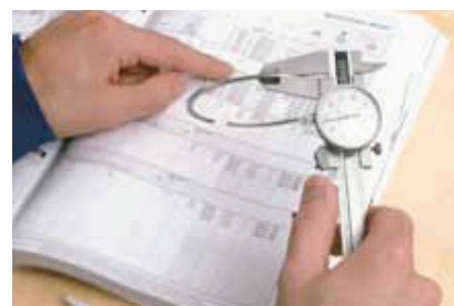
Checking with KS calliper with dial gauge, accuracy 0.01 mm KS art. no. 50 009 814
