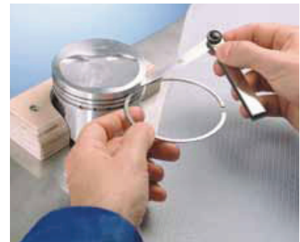
Measurement of the piston ring grooves with a feeler gauge. KS art. no. 50 009 824
